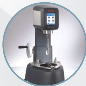
Vane rotor and universal container holder
